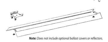
Part Numbers - 14060 and 14050: Converts an 8-foot, 2 Lamp T12 "strip-type" Light Fixture into an 8-foot, 4 Lamp T5 or T8 Light Fixture (Shown with optional P/Ns 14080, 14095 or 14096)
